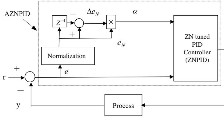
Fig. 1. Block diagram of the proposed AZNPID.
