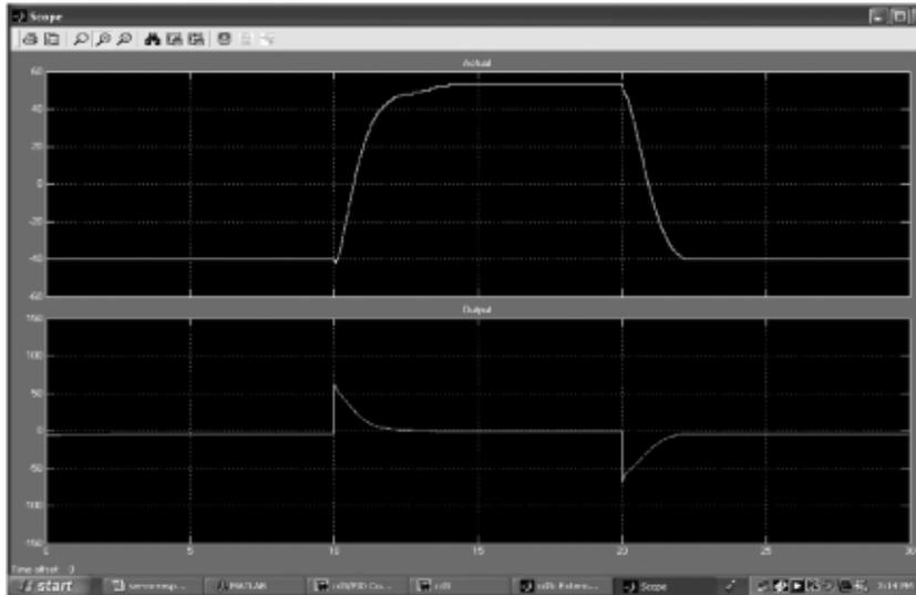
(a) Response and control action under ZNPID with 25% increased  $K_p$ .
