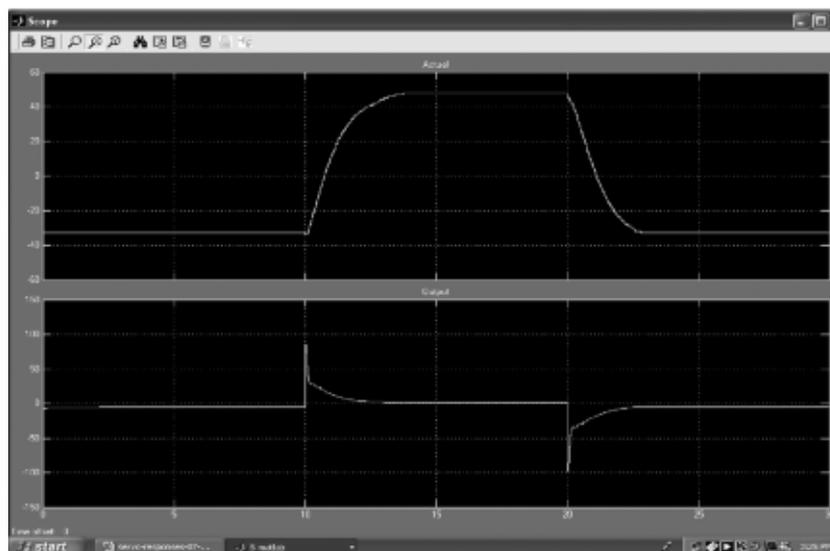
(b) Response and control action under AZNPID with 25% reduced  $K_p$ .
