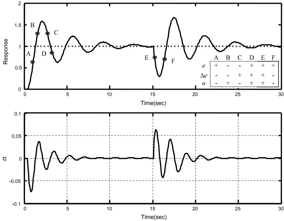
Fig. 4. Typical close-loop response of an under-damped second-order process (above) and its corresponding variation of the gain updating factor  $\alpha$  (below).
