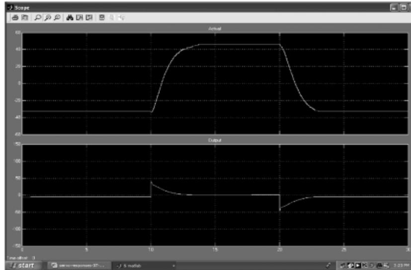
(a) Response and control action under ZNPID with 25% reduced  $K_p$ .
