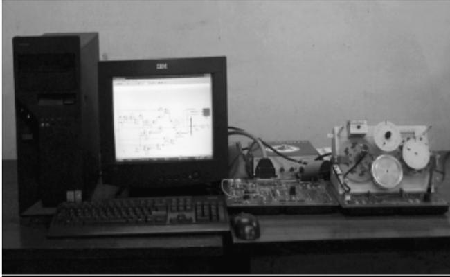
Fig. 10. Experimental setup of feedback digital servo process rig.
